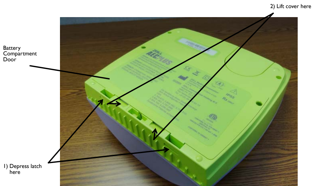
Figure 7: Removing the Battery Compartment Door
